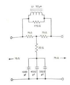
Figure 3: De-emphasis circuitry used in the receiver.
