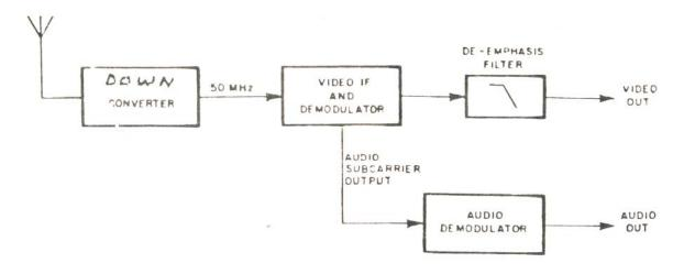
Figure 7: Block Diagram of a FM-ATV Receiver.
