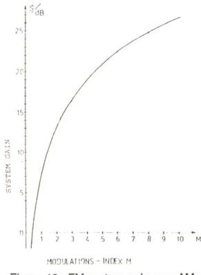
Figure 10: FM system gain over AM as a function of modulation index (M).
