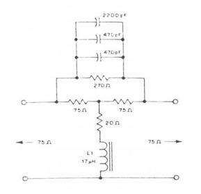
Figure 2: Pre-emphasis circuitry used in the FM-ATV transmitter.
