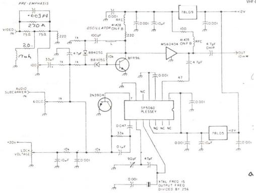
Figure 5: Exciter for generating FM-ATV.
